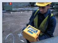
LMSxi - Contaminated land and landfill gas analyser
