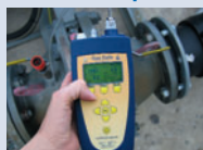
GFM400 - Biogas and landfill gas analysers
